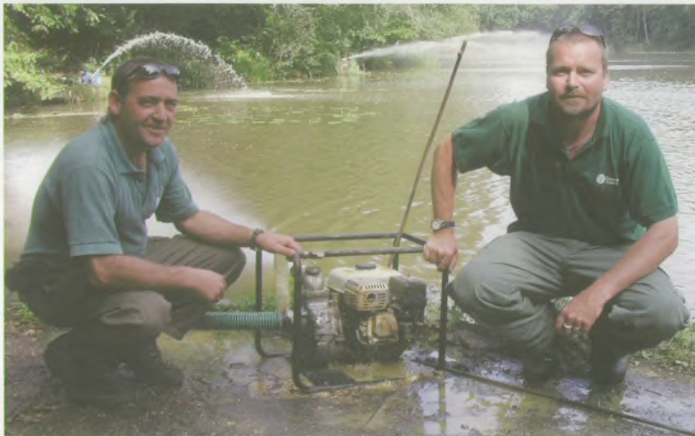
Raising the oxygen levels in a fishing lake - photo by Ray Kemp, Environment Agency
