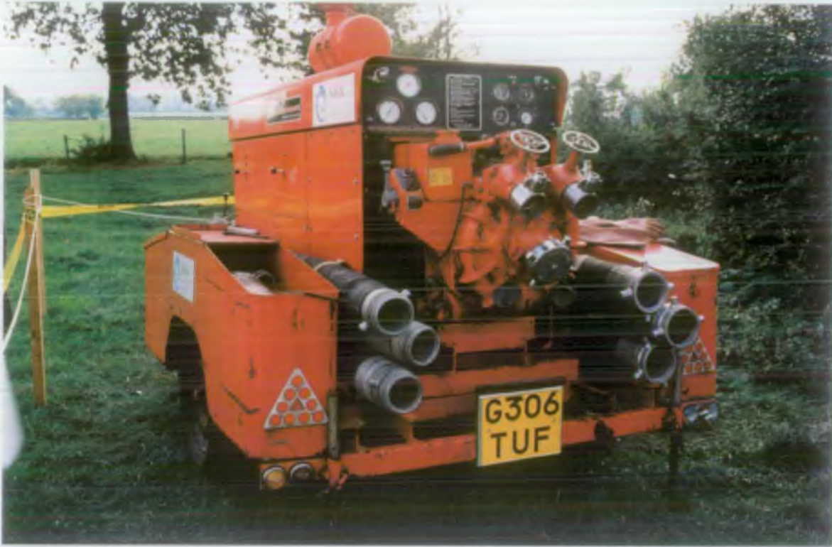
Plate 5: Godiva fire pump for BOC 'Vitox' oxygenation system
