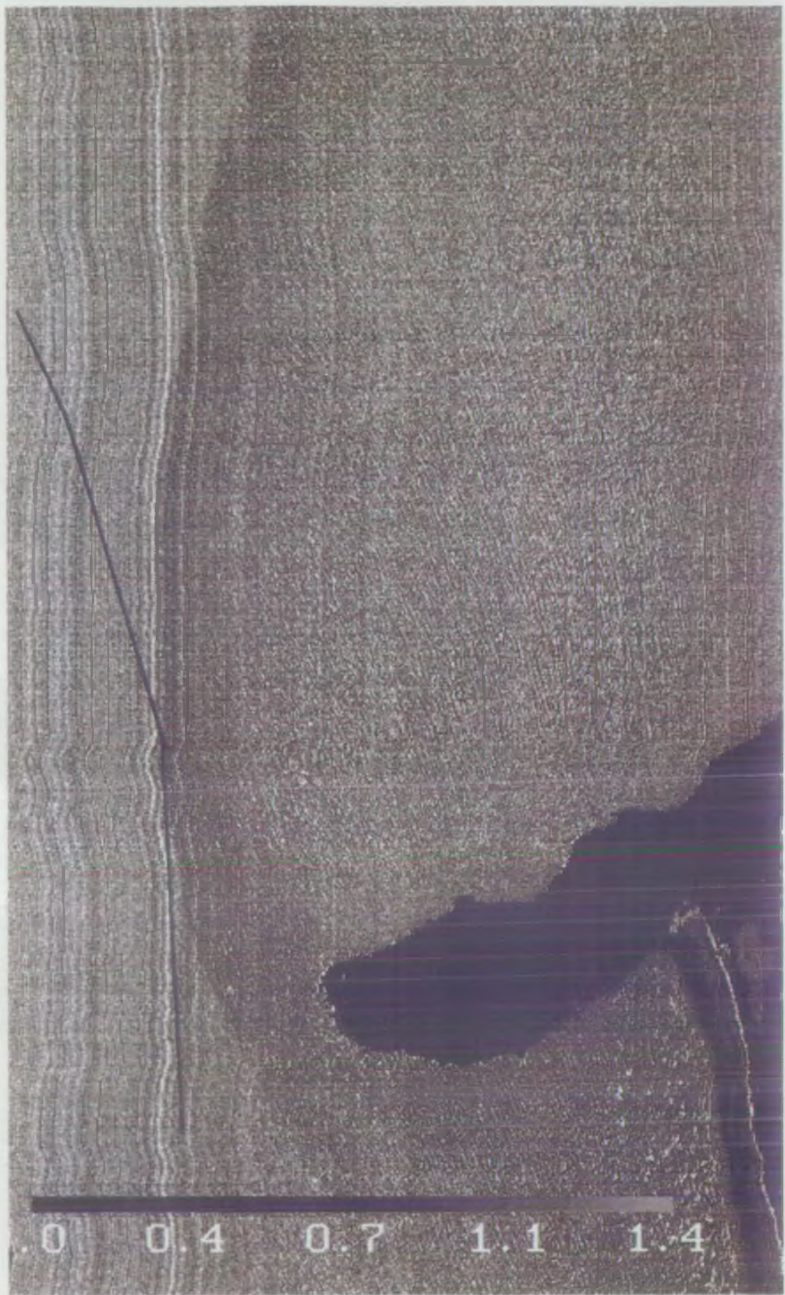
Appendix 14c: Variation in chlorophyll spatially around Brean Down, Weston-Super-Mare (15/05/93). Boat track data (black line) has been used to standardise it.
