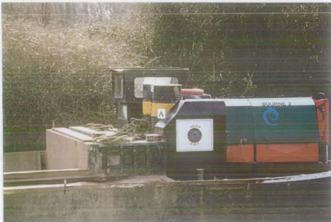
Picture 8 Dredger "Bourne 2" on the river Medway below Oak Weir. A - fuel oil drums carried, unsecured and unbanded.
