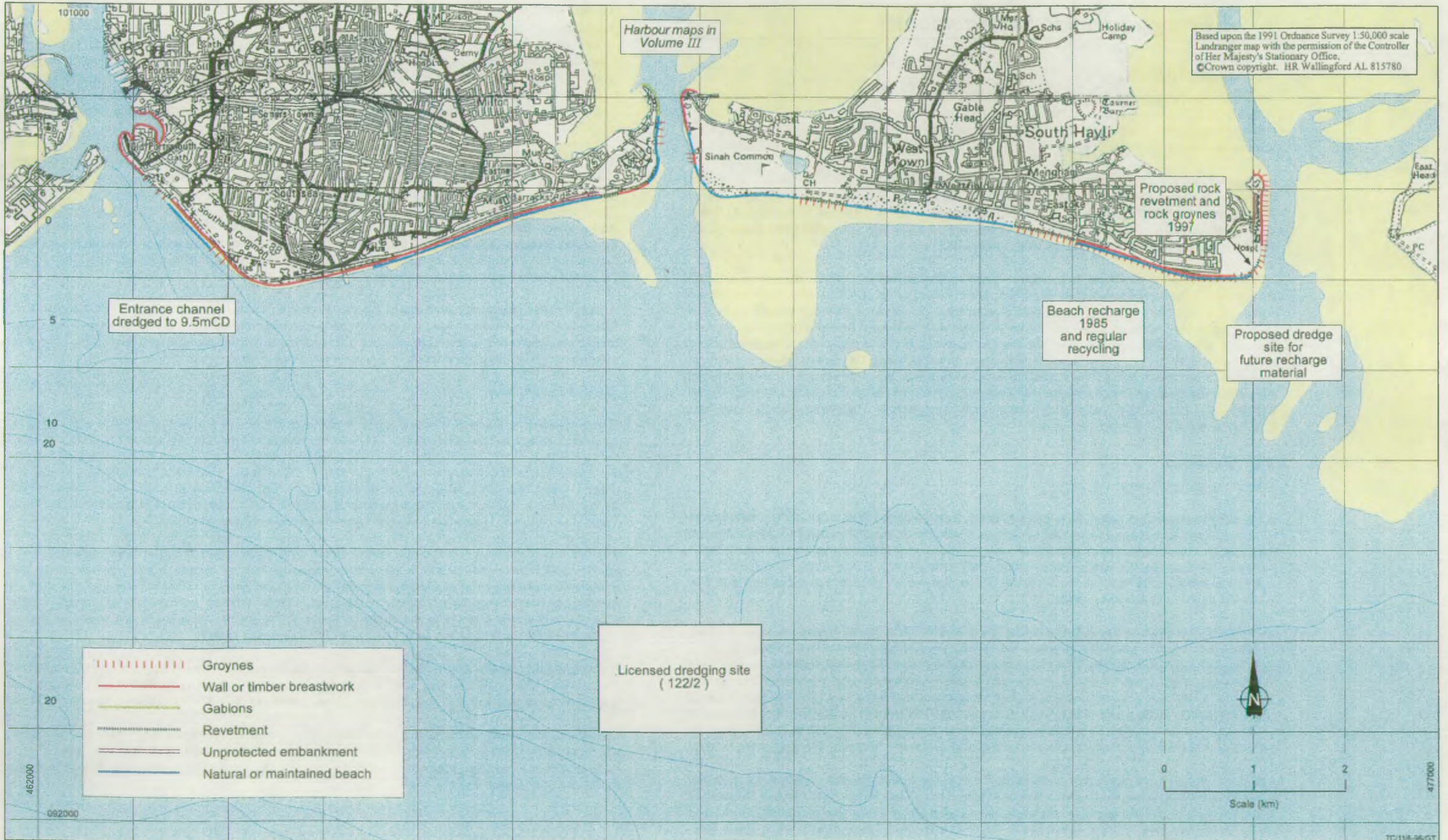
Existing shoreline defences - Hayling and Portsea Islands
