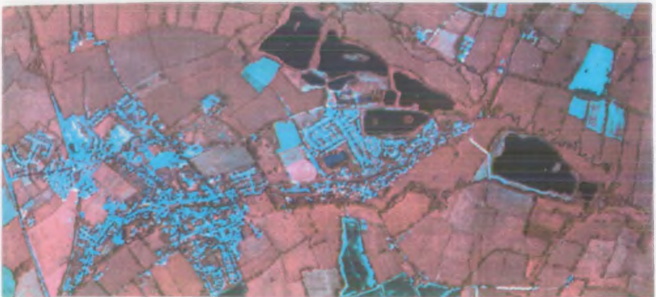
Figure 5.1 A comparison of three different waveband combinations (simulated true colour, with near infrared and with thermal bands) from digital Airborne Thematic Mapper data (see text); the original sheets have been reduced from 1:10,000 to approx. 1:20,000 to show the range of variation in colour and thus interpretation, available.
