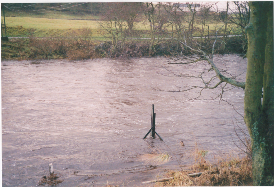
Middleton in Teesdale upstream transducer rack under high flow conditions
