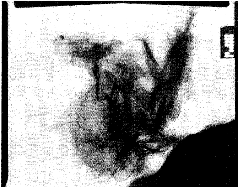
Figure A23. Reference Backfill Groundwater water A, 85°C, 20 months: The large electron-dense region to the lower right is a calcite grain. The large hexagonal plate (and the dark elongated shapes, which may be plates edge-on) are of pure Fe. The smaller hexagonal plates forming on these plates are unknown composition but may be portlandite or an AFm phase. Magnification x 60,000.
