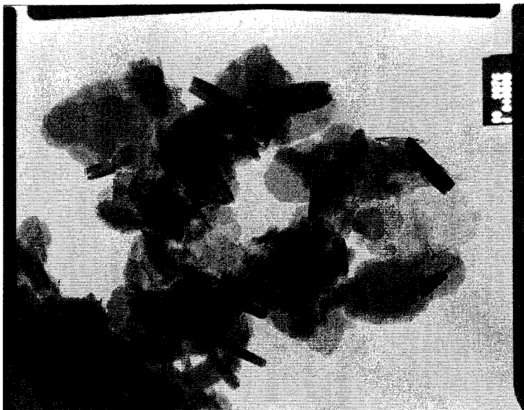
Figure A8. 60 pfa: 40 OPC Deionised water, 85°C, 20 months: Stubby prisms of an Fe phase with hexagonal plates (possibly of portlandite). Magnification x 46,000.
