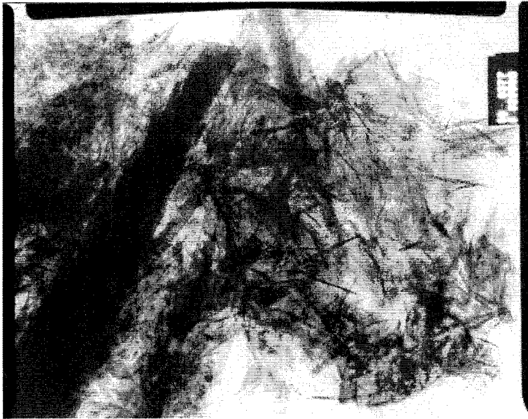
Figure A21. 60 pfa: 40 OPC Groundwater water A, 85°C, 20 months: A few coarse zeolite prisms amongst CSH sheets (whose curled up edges appear as electron-dense spikes), some finer grained prismatic zeolites and a few tiny patches of gel. Magnification x 28,000.
