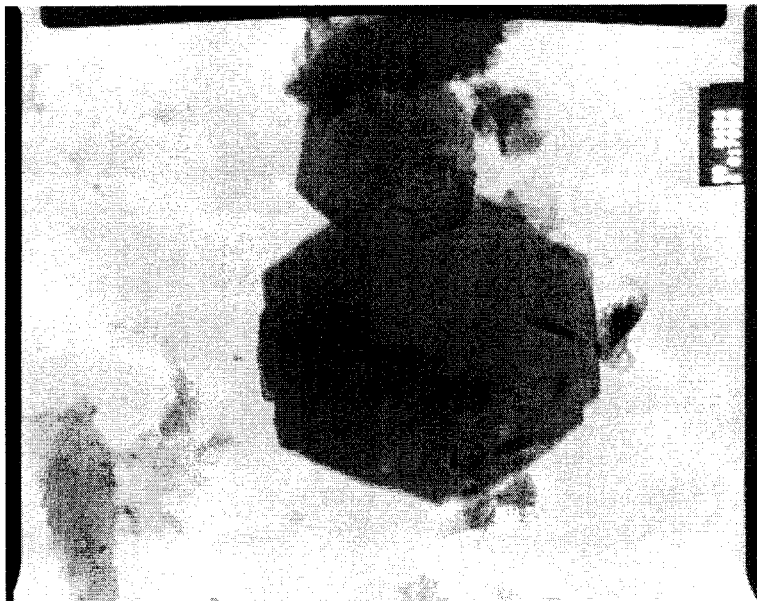
Figure A27. Reference Backfill Groundwater water A, 85°C, 20 months: Coarse hexagonal plates of pure Fe. Magnification x 17,000.
