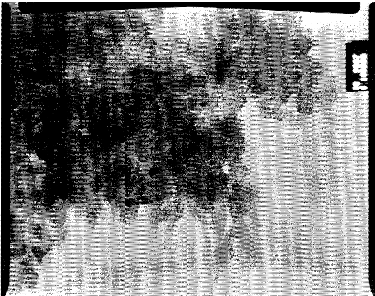
Figure A14. 60 pfa: 40 OPC Deionised water, 85°C, 20 months: Typical mixture of needles and hexagonal plates. Magnification x 100,000.
