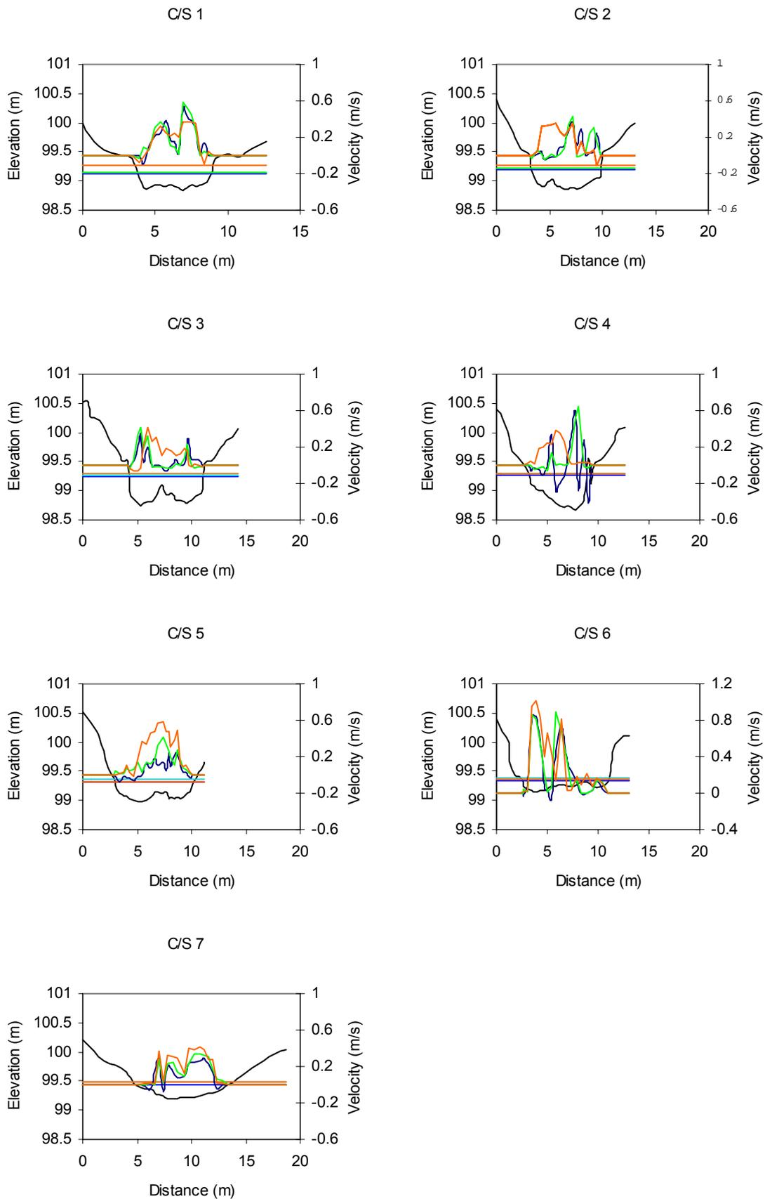
**Figure C4.1 West Stafford: cross section plots showing water surface levels and velocities**
