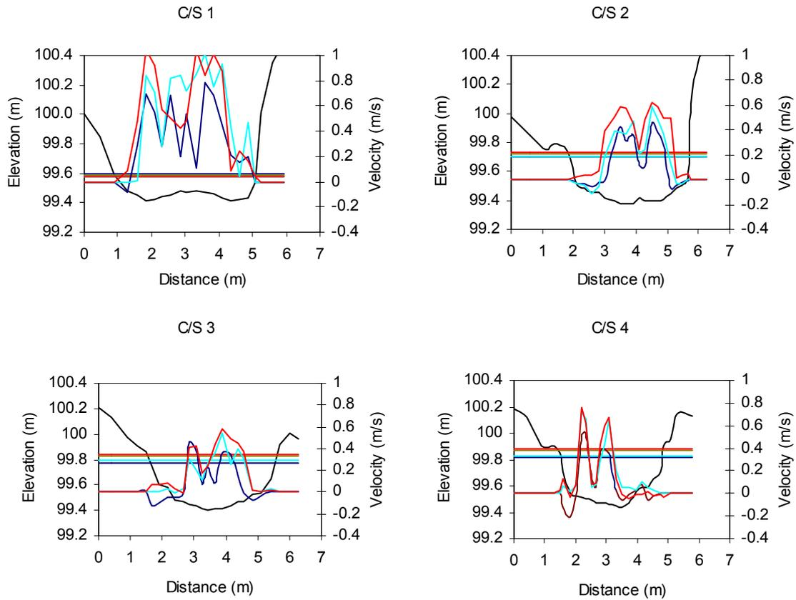
**Figure C4.5 West Stafford Carrier: cross section plots showing water surface levels and velocities**
