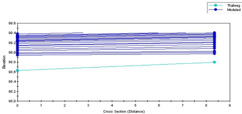
Figure 5.6: River Walkham (lower site): simulated water surface levels.
