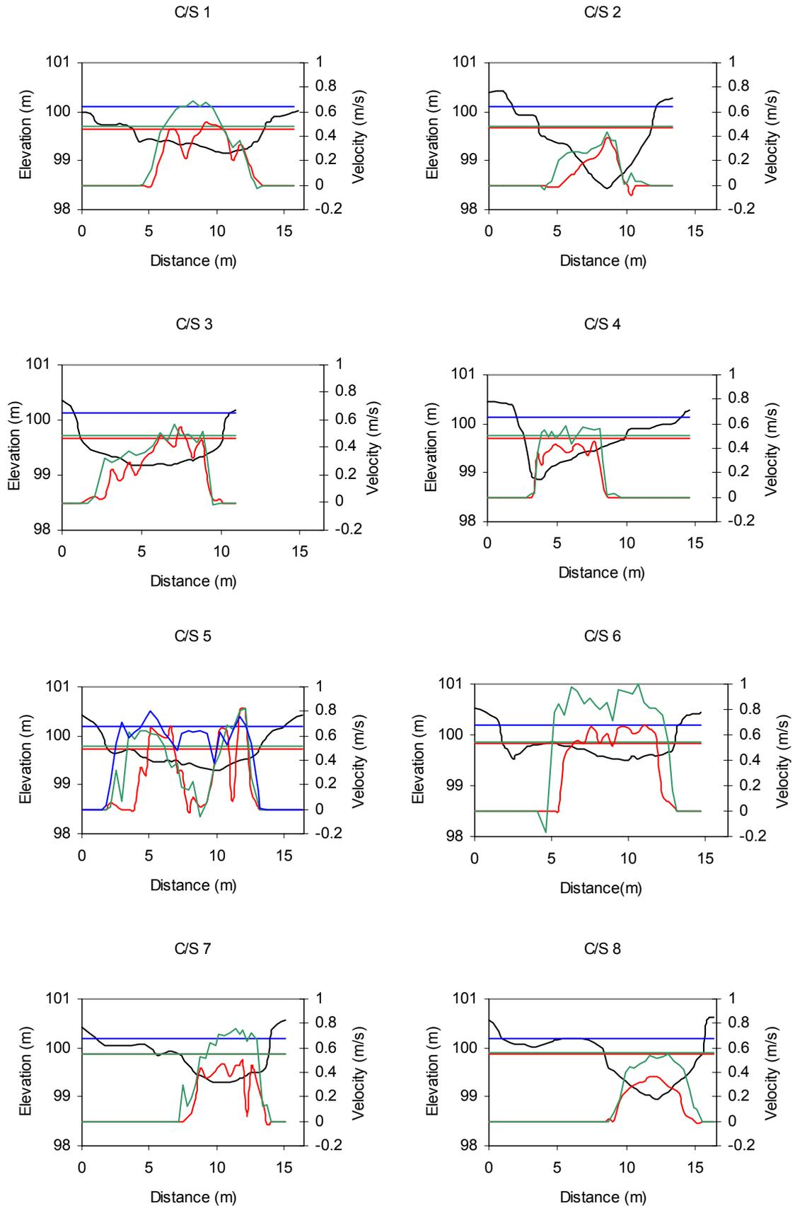
**Figure C2.1: River Piddle: cross section plots showing water surface levels and velocities**
