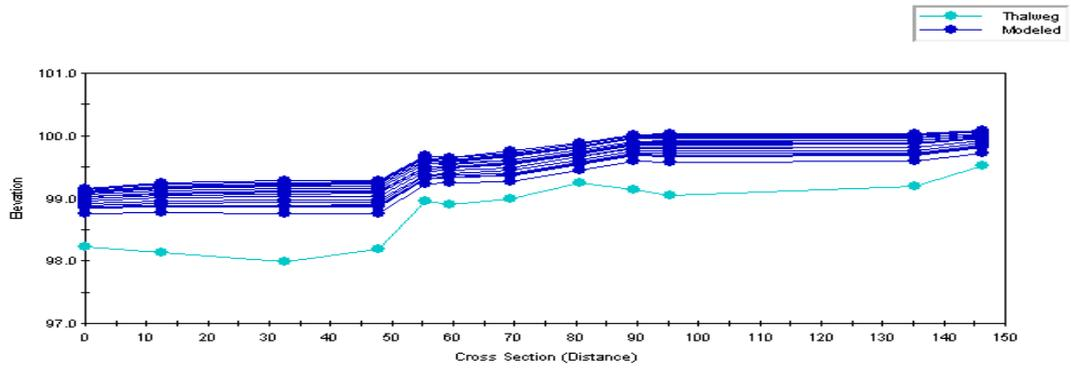
Figure C3.3 River Senni: simulated water surface profiles
