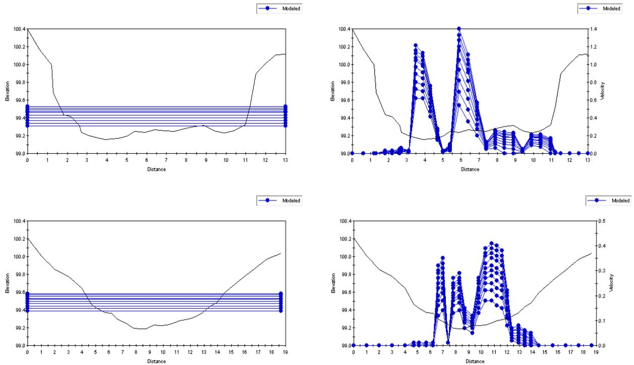
**Figure C4.4 West Stafford: simulated water surface levels and velocities (cont)**
