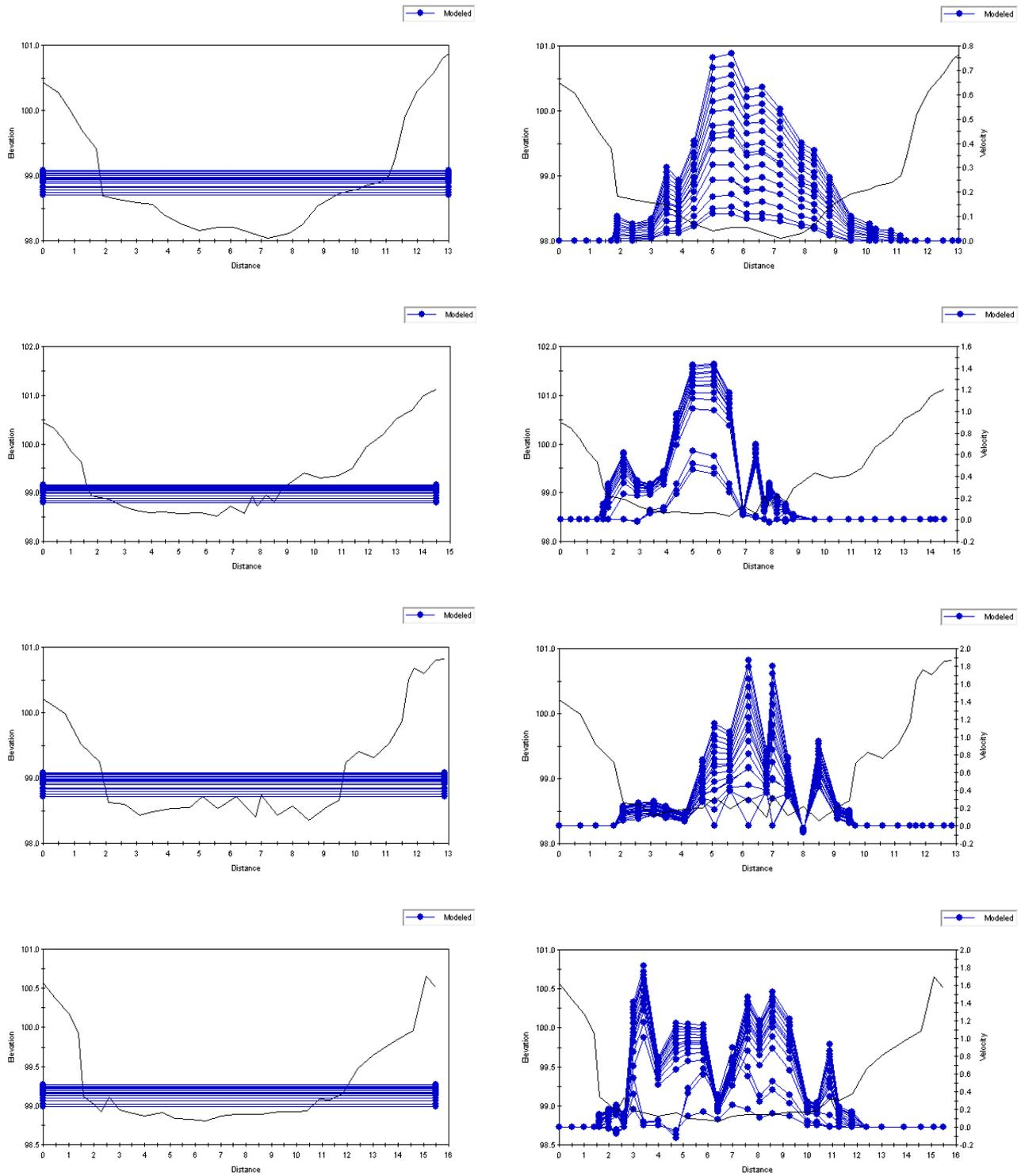
**Figure C1.8: River Walkham (upper site) simulated water surface levels and velocities (cont).**
