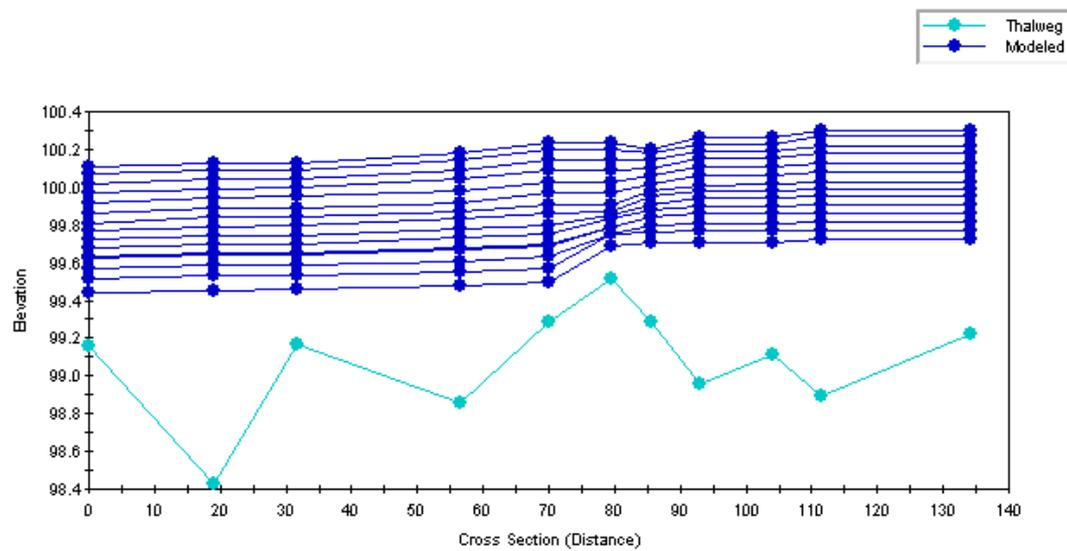
**Figure C2.3 River Piddle: simulated water surface profiles**
