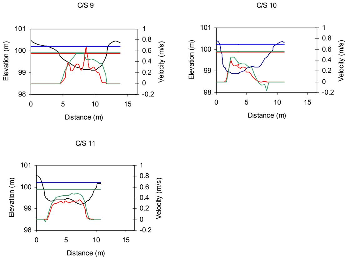
**Figure C2.1 (continued) River Piddle: cross section plots showing water surface levels and velocities**
