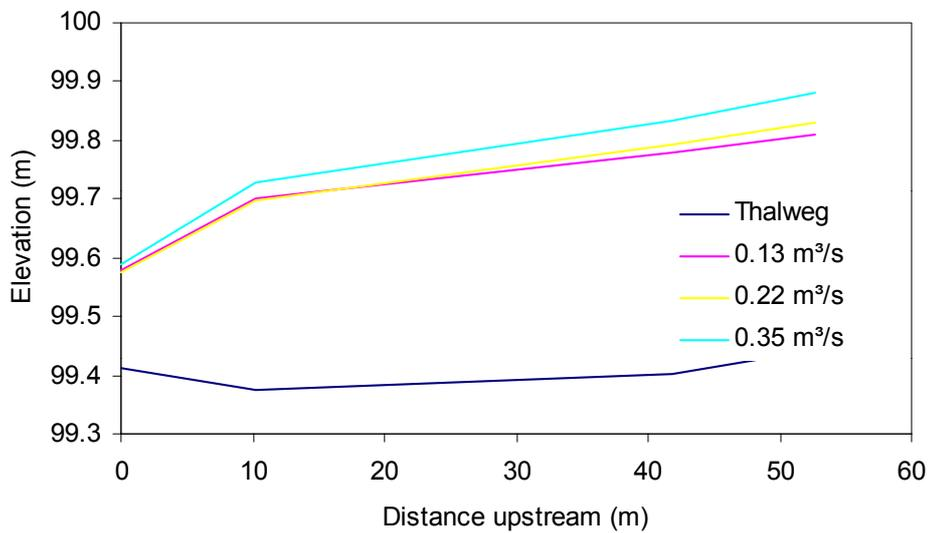
**Figure C4.6 West Stafford Carrier: measured water surface profiles**
