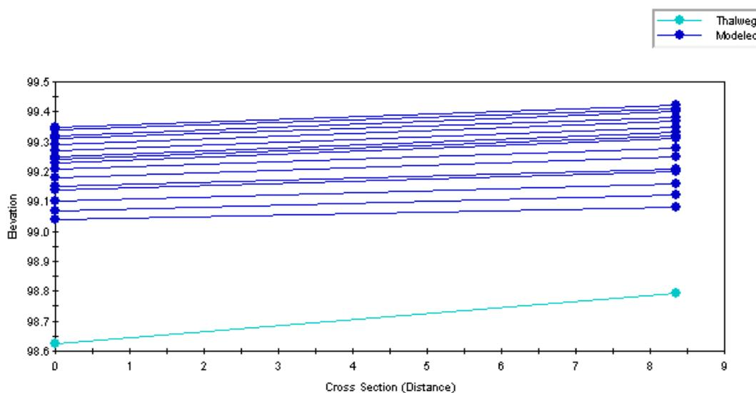
**Figure C1.5: River Walkham (lower sites): simulated water surface profiles**
