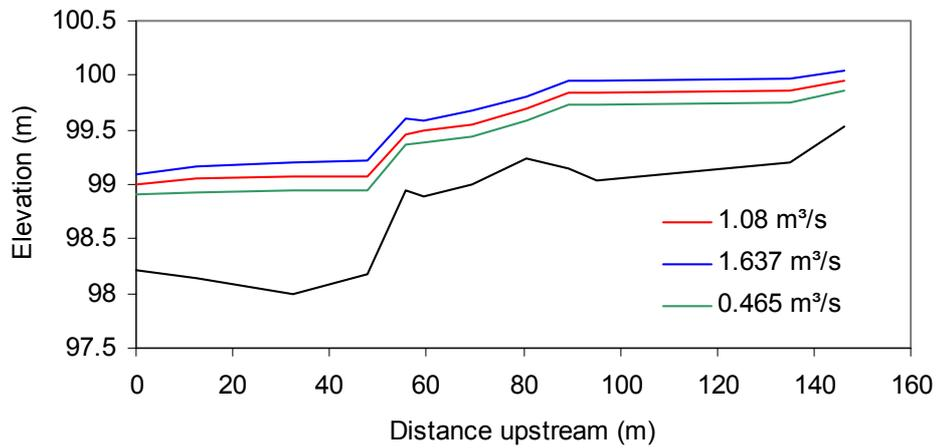
**Figure C3.2. River Senni: measured water surface profiles**
