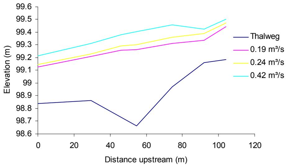
**Figure C4.2 West Stafford: measured water surface profiles**
