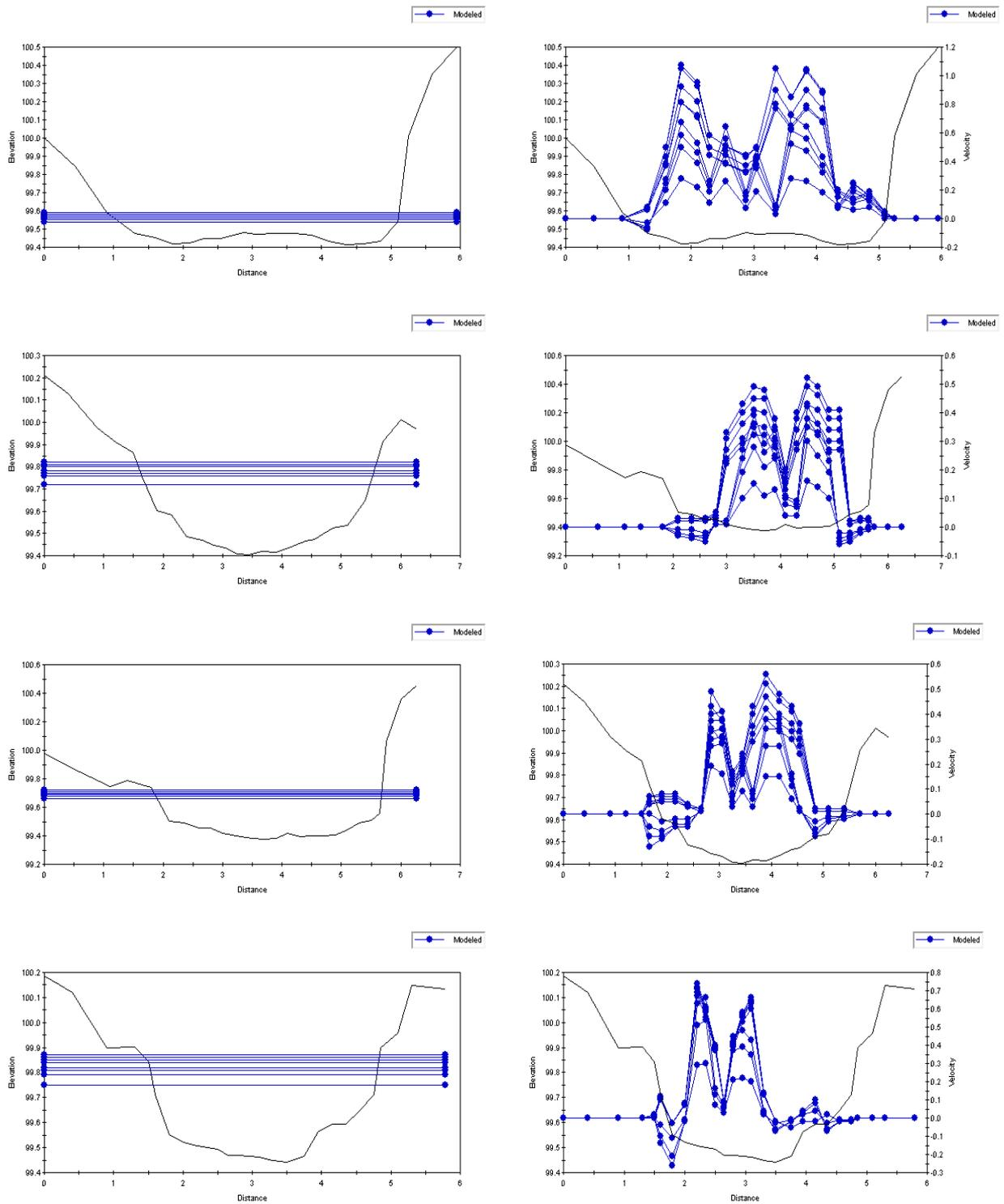
**Figure C4.8 West Stafford Carrier: Simulated water surface levels and velocities**
