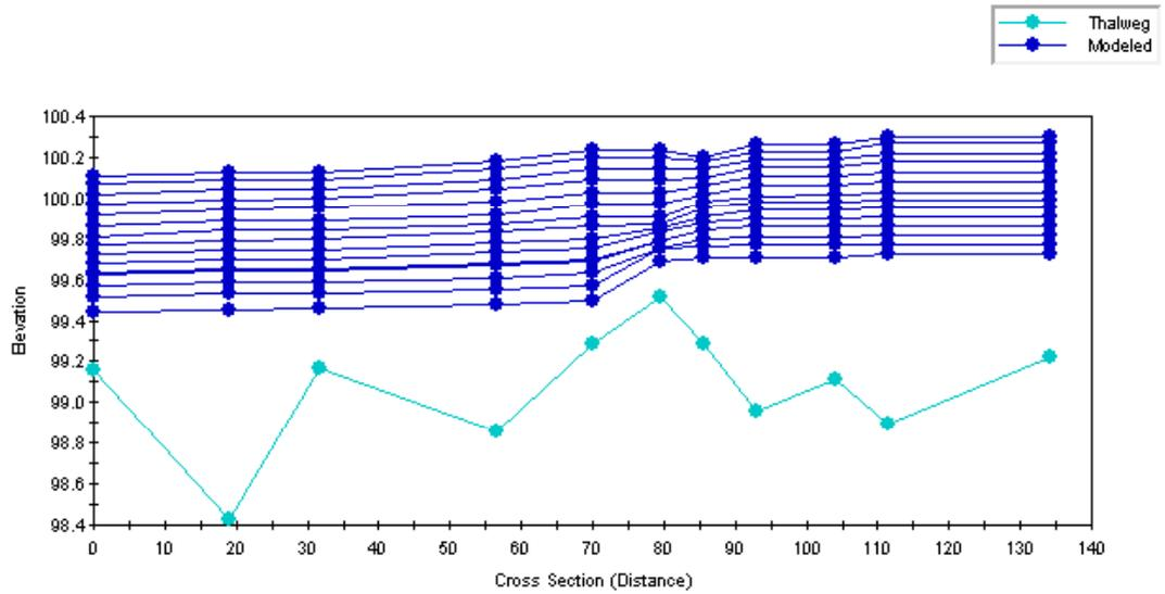
**Figure 5.10: River Piddle: simulated water surface levels.**
