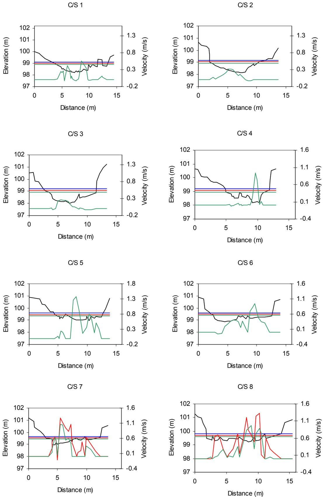
**Figure C3.1 River Senni: cross section plots showing water surface levels and velocities**
