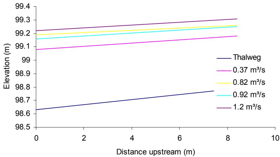
**Figure C1.3: River Walkham (lower site): measured water surface profiles.**
