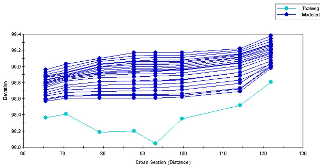
**Figure C1.6: River Walkham (upper sites): simulated water surface profiles.**
