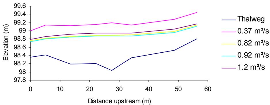
**Figure C1.4: River Walkham (upper site): measured water surface profiles.**
