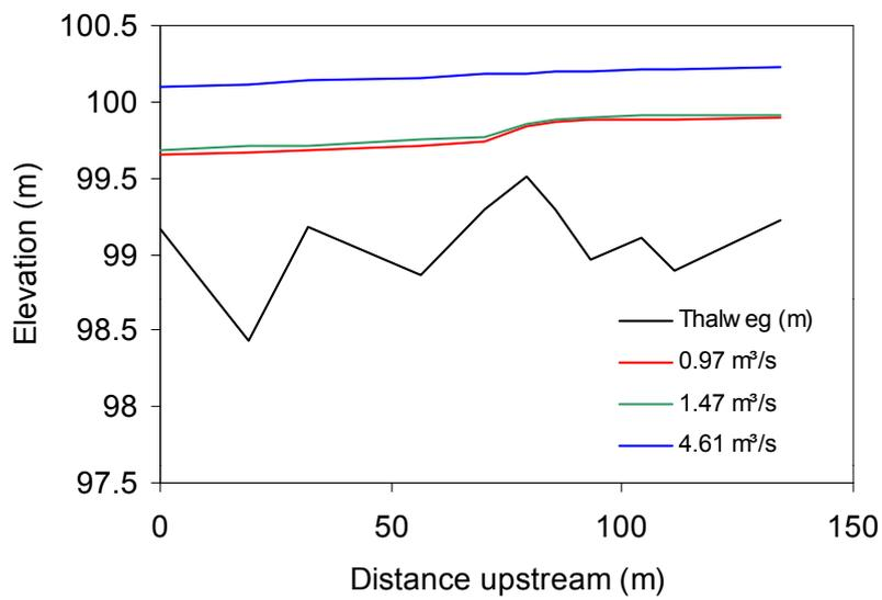
**Figure C2.2. River Piddle: measured water surface profiles.**
