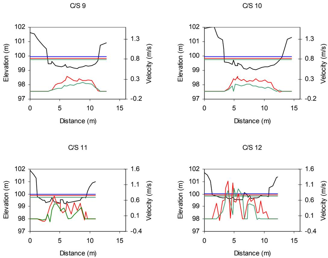
**Figure C3.1 (continued) River Senni: cross section plots showing water surface levels and velocities**
