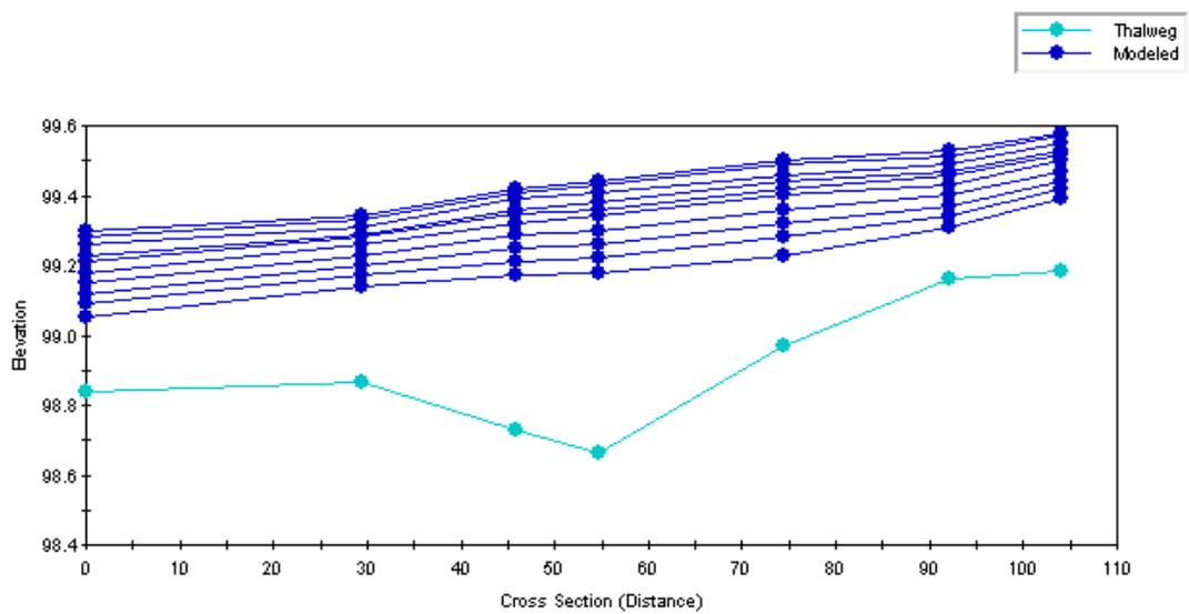
**Figure C4.3 West Stafford: simulated water surface profiles.**
