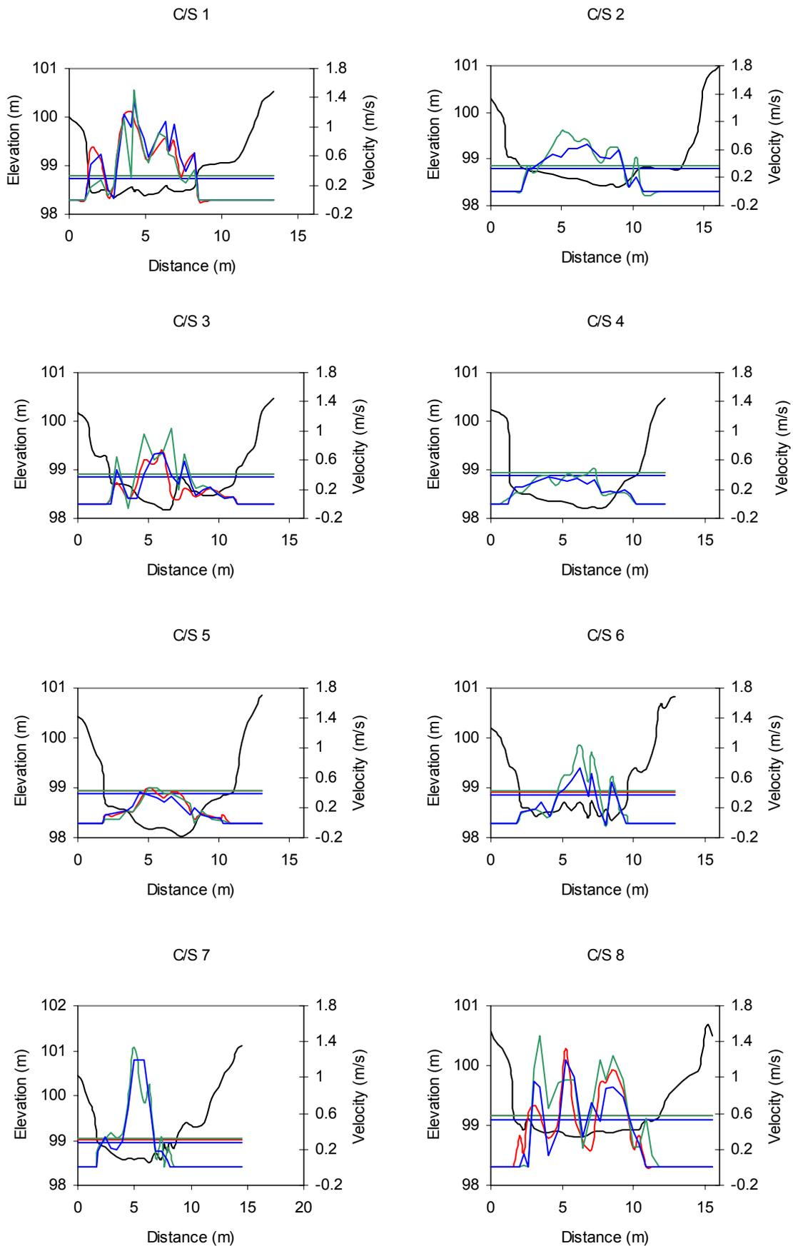
**Figure C1.2: River Walkham (upper site): cross section plots showing water surface levels and velocities**
