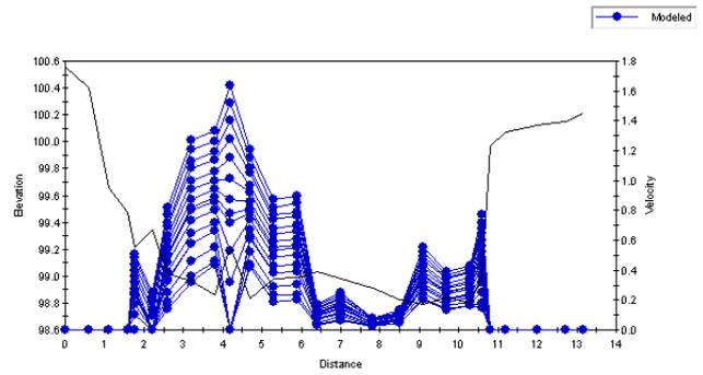
**Figure C1.7: River Walkham (lower site): simulated water surface levels and velocities.**
