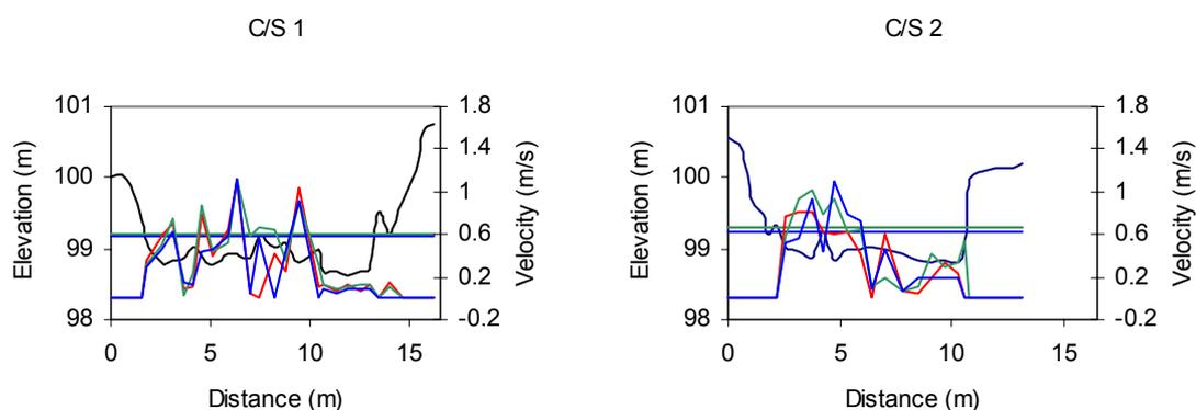
Figure C1.1: River Walkham (lower site): cross section plots showing water surface levels and velocities
