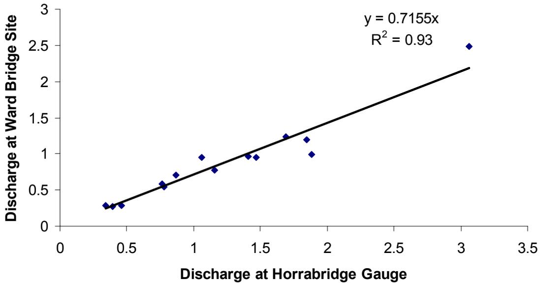
**Figure 7.2: Regression relationship between discharge at Horrabridge (continuously-gauged) and at Ward Bridge (spot-gaugings)**
