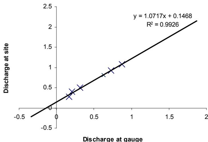
**Figure 7.4: Regression relationship between discharge at Pont-hen-Hafod (continuously-gauged) and at Abersenny (spot-gaugings)**
