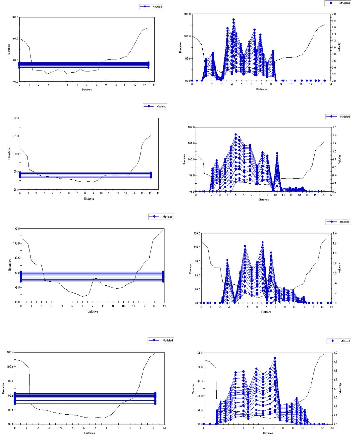
**Figure C1.8. River Walkham (upper site): simulated water surface levels and velocities**
